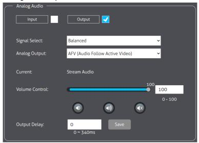
Configure the 5-pin Audio In/Out terminal as an analog audio output.
