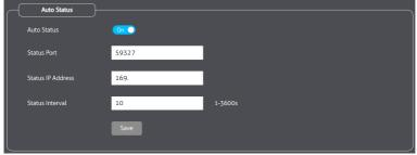
When enabled, the unit sends status information to the network whenever the status changes and at a user defined time interval.
