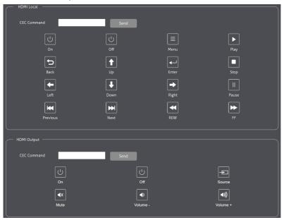
**HDMI Local:** Press the buttons or send HEX CEC commands to control the HDMI input display.
