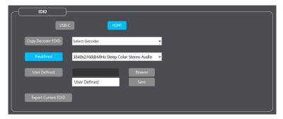
Configure the EDID for the USB-C and HDMI inputs.
