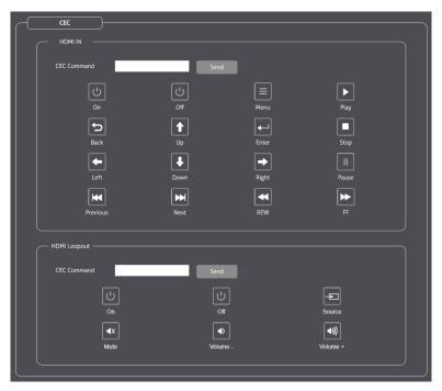
**HDMI IN:** Press the buttons or send HEX CEC commands to control the HDMI input display.
