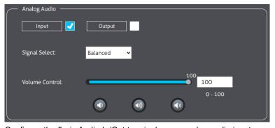
Configure the 5-pin Audio In/Out terminal as an analog audio input.
