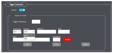
When enabled, the web UI sends predefined data to a specified IP address upon event occurrence. Supports exporting and importing trigger command configurations.
