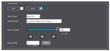
Configure the 5-pin Audio In/Out terminal as an analog audio output.
