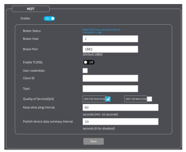
When enabled, configure the Broker Host (IP address), Broker Port, QoS, and Keep-Alive Interval. You can also enable TLS/SSL and user credentials if necessary.
