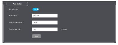
When enabled, the unit sends status information to the network whenever the status changes and at a user defined time interval.
