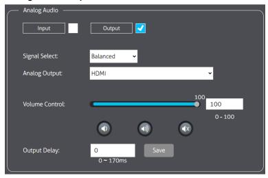
Configure the 5-pin Audio In/Out terminal as an analog audio output.
