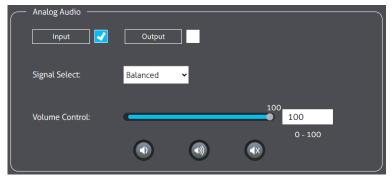
Configure the 5-pin Audio In/Out terminal as an analog audio input.
