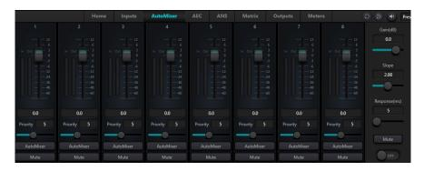
the level of non-active audio signal sources, such as a microphone, while simultaneously adjusting the level of the active sources accordingly to maintain a desired target gain. This eliminates the need for live mixing of audio sources.
