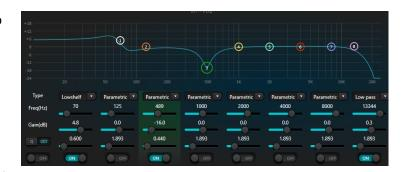
the opposite. Lowpass adds a cut off point where all frequency content above the cut off point will be removed. The highpass does the opposite to a lowpass filter.
