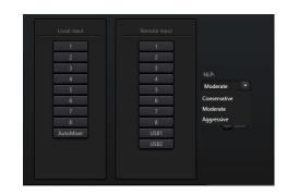
**NLP:** Non Linear Processing defines the length of time the reference (or remote) signal will be compared with the program (or local) signal and used for echo estimation. If the length of the echo is greater than the NLP value the echo will still be heard in the program signal. The following presets corresponds to the milliseconds in the columns below:
