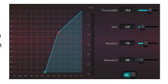
**Ratio:** The gain curve, or amount of expansion, is defined by the ratio value.
