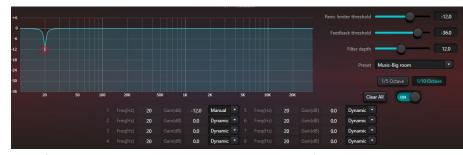
above the Panic Threshold will be detected as feedback. When a signal crosses above any of the following will occur to attenuate the feedback:
